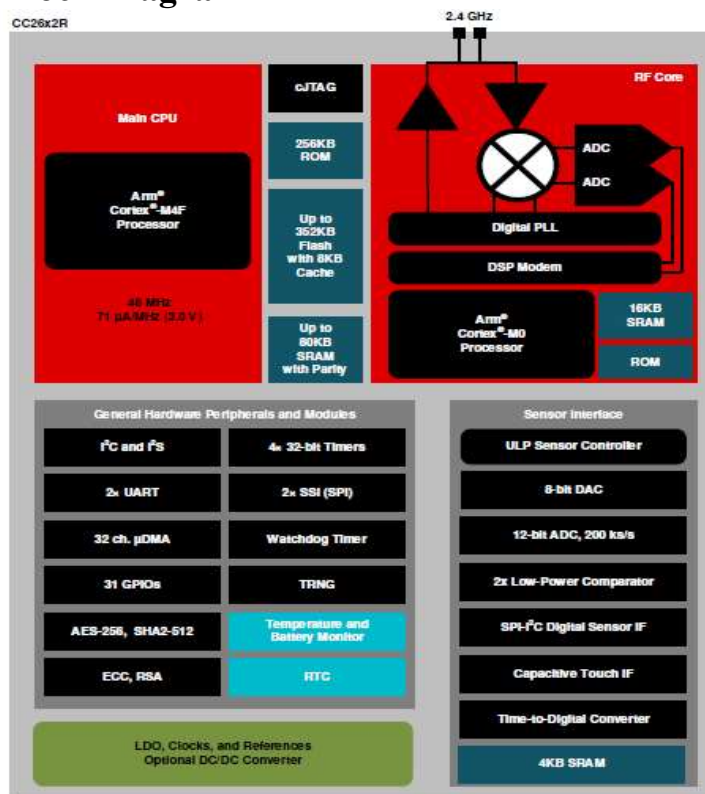
Figure 1-1. CC2642R Block Diagram
