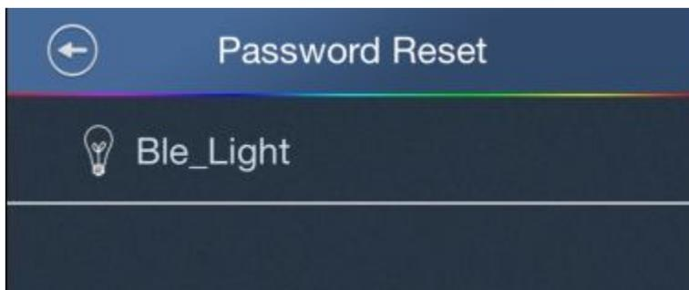
(3) Cut the lights' power and then power on, click the light's name in 30S and there will Pop-up reset password box. Input password and click Confirm, the system will tip password reset successful.
